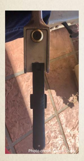
I strung my bow to give the plates time to become secure while the epoxy dried. You can use clamps too. The plates I ordered fit properly and the limbs appeared they would be straight once I strung the bow using a bow stringer. I also used the new ILF limb bolts I purchased and I greased threads up with white lithium grease and ran the limb bolts in and out a couple of times. Make sure you are using ILF system limb bolts. You can get ILF limb bolts as a kit.
