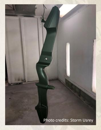
Make sure to degrease the riser before painting and use a lint free cloth to wipe down. I recommend putting in the older limb bolts and any bolts in any of the holes to protect your threads. Primer, paint and clear coat your riser (several coats will be required). I used a matte paint as I may choose to hunt with my recurve too. After the paint cures you are ready to put your bow back together and shoot.
