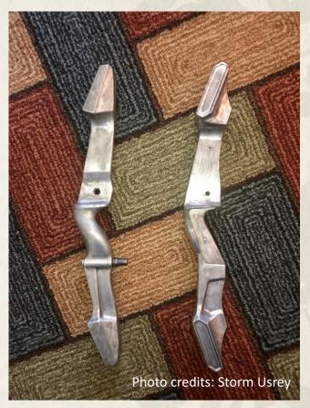
I opted to take the old paint off the two risers I obtained using paint stripper. Make sure to wear the appropriate safety equipment and do this in a well ventilated area. It's a good idea to keep old limb bolts to use during painting. I used a Dremel with wire and nylon brush attachments to assist in paint removal.
