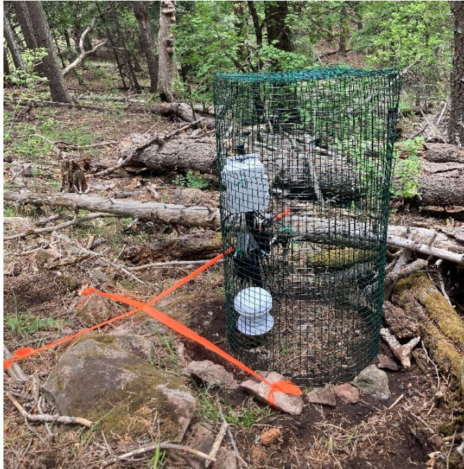
Figure 3. HOBO weather station monitoring environmental variables in a Sacramento Mountain salamander ( A. hardii ) demography plot. Orange flagging crosses above the location of an instrumented rock.
