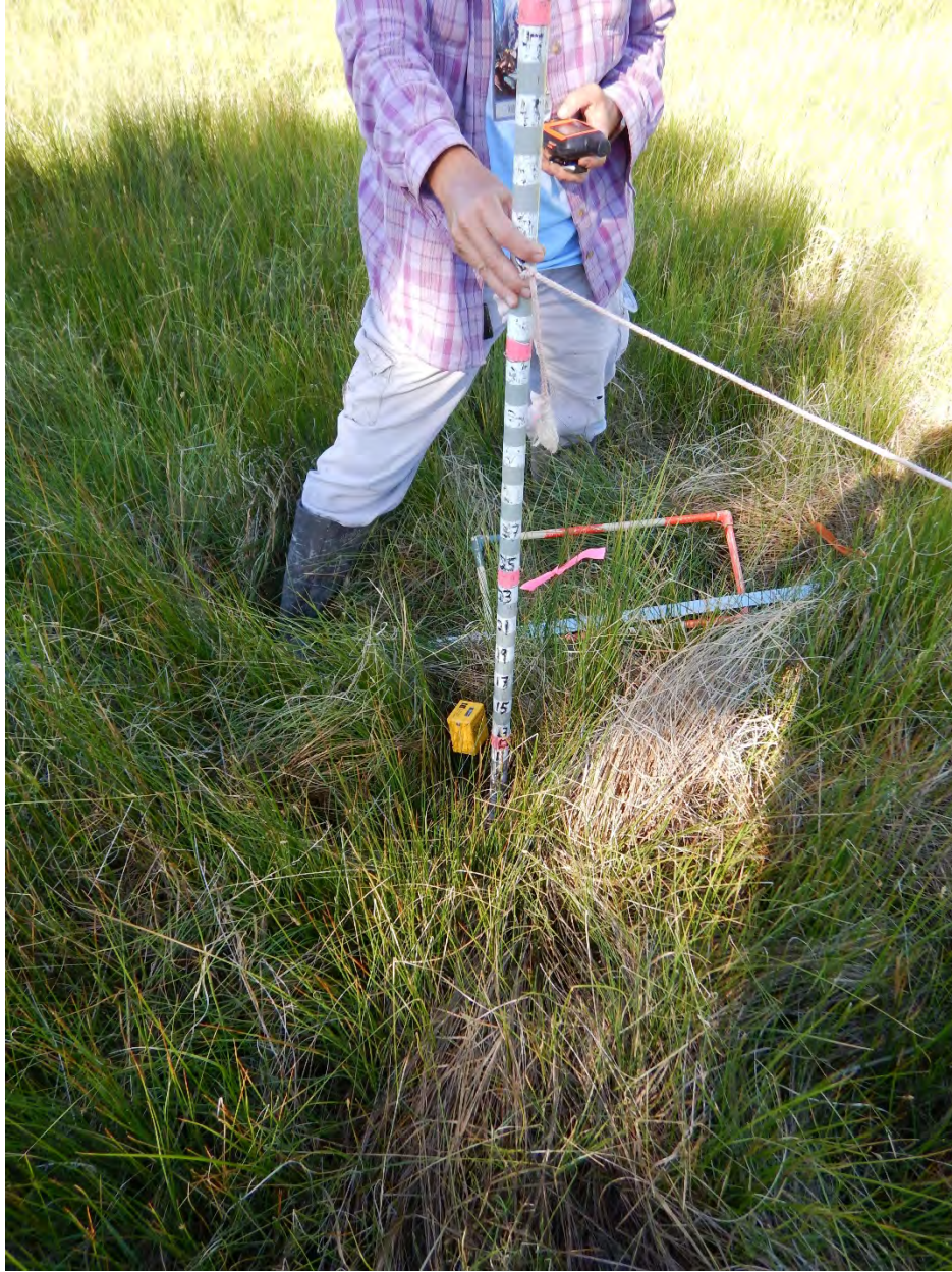
Measuring habitat at Funderburg Spring with Robel pole, Daubenmire frame, soil moisture meter, and meter ruler. The Robel pole provides the best measurement of montane vole habitat.
