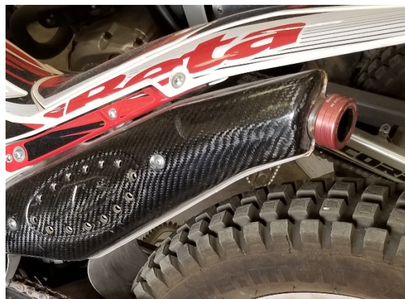
Add-on (red) spark arrester on Beta trials motorcycle
