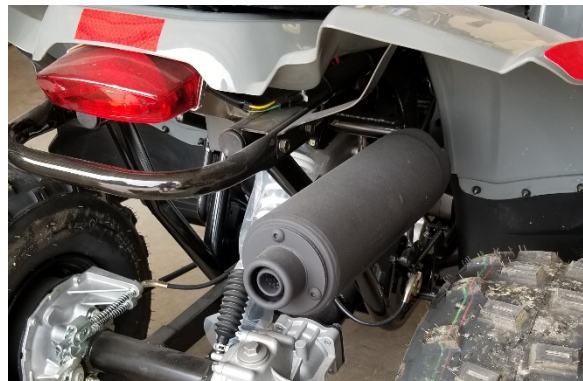
Screen type spark arrester/muffler on Polaris ATV
