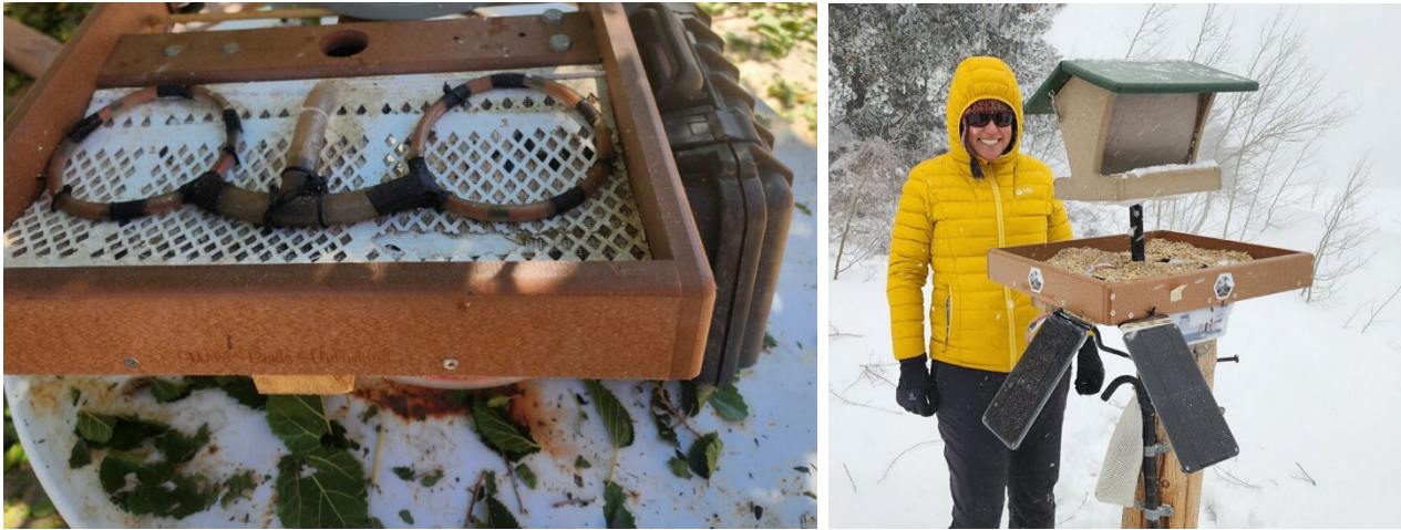
RFID reader antenna coils within feeder tray (left) and fully assembled feeder with additional metal layer added atop coils for protection and covered with seed (right).
