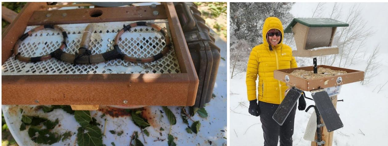
*Radio frequency identification (RFID) reader antenna coils within feeder tray (left) and fully assembled feeder with additional solid plastic layer added atop coils for protection from elements and rodents and covered with seed (right). Photos by Corrie Borgman, USFWS.*
