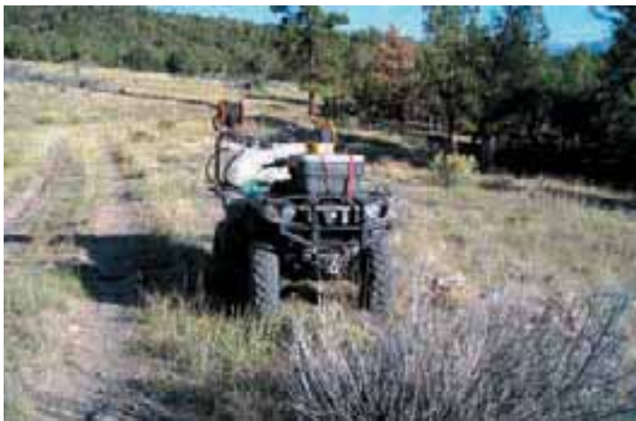
Figure 33. Sprayer-mounted all terrain vehicles or aircraft are often the most effective ways to distribute herbicides across rangelands. (Left photo by Dave Hale/CDOW; right photo by Bruce Watkins/CDOW).
