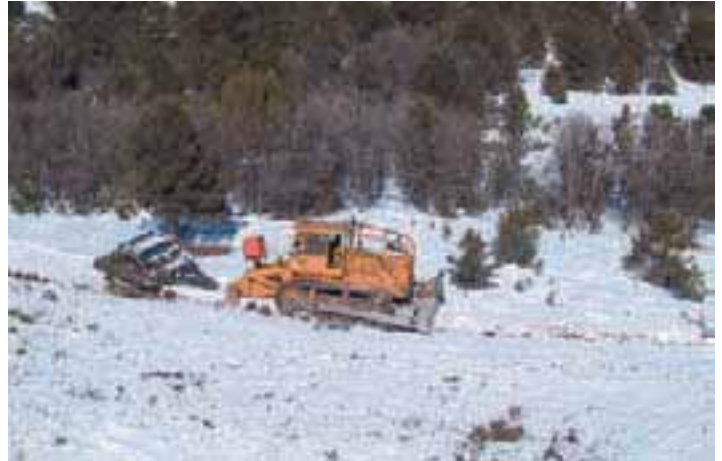
Figure 19. Roller choppers offer a more affordable method of mechanically treating large areas. (Photo by Bruce Watkins/CDOW).
