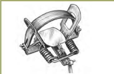
**Figure WC9b.** Unmodified jaw coil-spring trap (closed)
