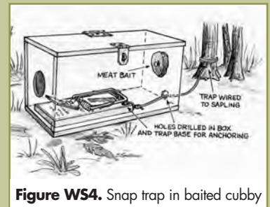
**Figure WS4.** Snap trap in baited cubby
