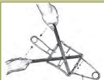
**Figure SKF3a.** Using setting tool
