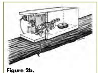
Bodygrip trap in baited cubby with pan trigger
