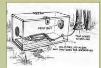
Figure WS4. Snap trap in baited cubby
