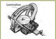
Figure RF6a. Laminated jaw trap
