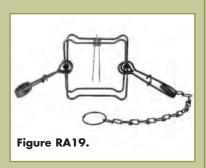
Height of trap window: 6 1/8 inches Width of trap window: 6 inches Diameter of frame wire: 3/16 inch Diameter of spring wire: 3/16 inch Additional clamping bar: None
