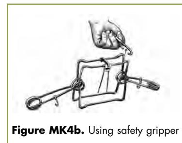
**Figure MK4b.** Using safety gripper
