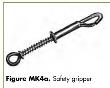
**Figure MK4a.** Safety gripper
