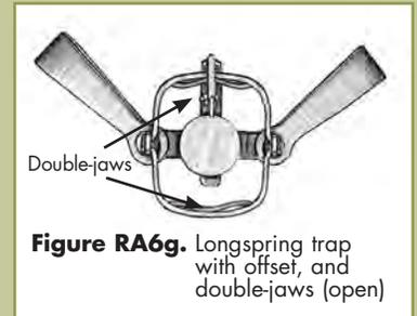
**Figure RA6g.** Longspring trap with offset, and double-jaws (open)
