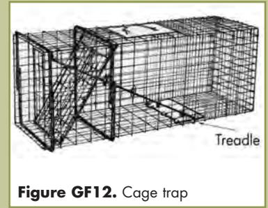
Figure GF12. Cage trap
