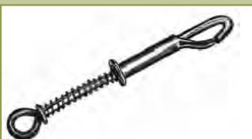
**Figure BV5a.** Safety gripper
