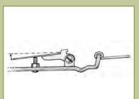
Figure 15b. Pan stop, closed position
