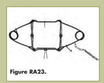
Height of trap window: 6 1/8 inches Width of trap window: 7 3/4 inches Diameter of frame wire: ¼ inch Diameter of spring wire: ¼ inch Additional clamping bar: None
