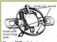
Figure BV7a. Coil-spring trap
