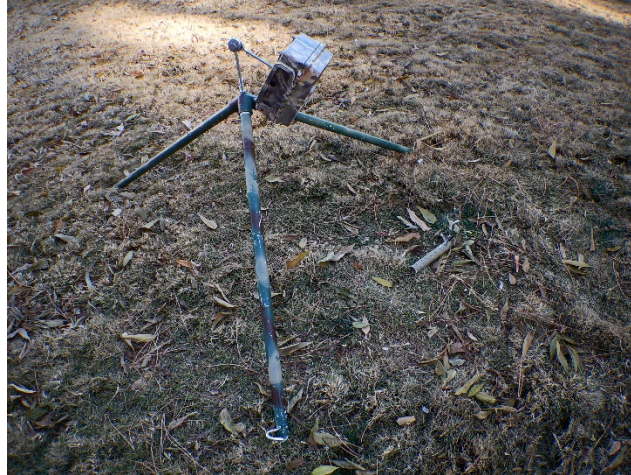
Figure 4. Camera mounting stand and bait tube. The stand and bait tube are anchored to the ground with tent stakes.
