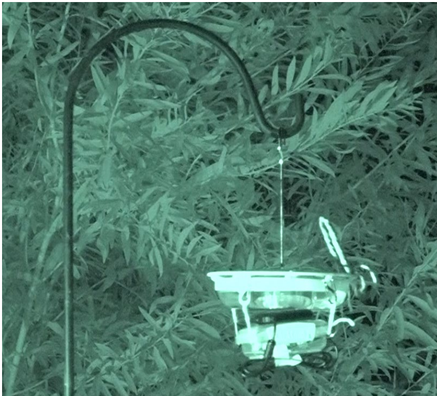
Figure 6. PIT tag detection system and modified hoop antenna deployed in the field. Photo: Mallory Davies.
