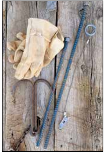
Left to right: Drag, 18" stake, 24" stake and earth anchor (disposable type). NMDGF photo.
