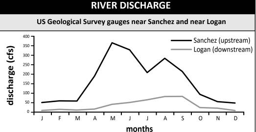
Mean monthly discharge at two stream gauges from 1963, when Ute Reservoir was completed, until 2014. Discharge is measured in cubic feet per second (cfs). Sanchez gauge is located upstream of Conchas Reservoir, so discharge is not influenced by the major dams. Logan gauge is downstream of Ute Reservoir where discharge is reduced. Peaks in discharge are from spring run-off and summer monsoon rain. Pulses of high flow are important cues for reproduction in some fish species.
